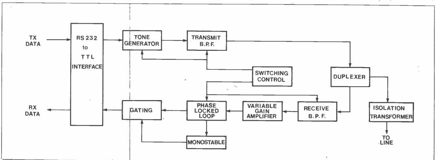
Figure 1. Modem block diagram
