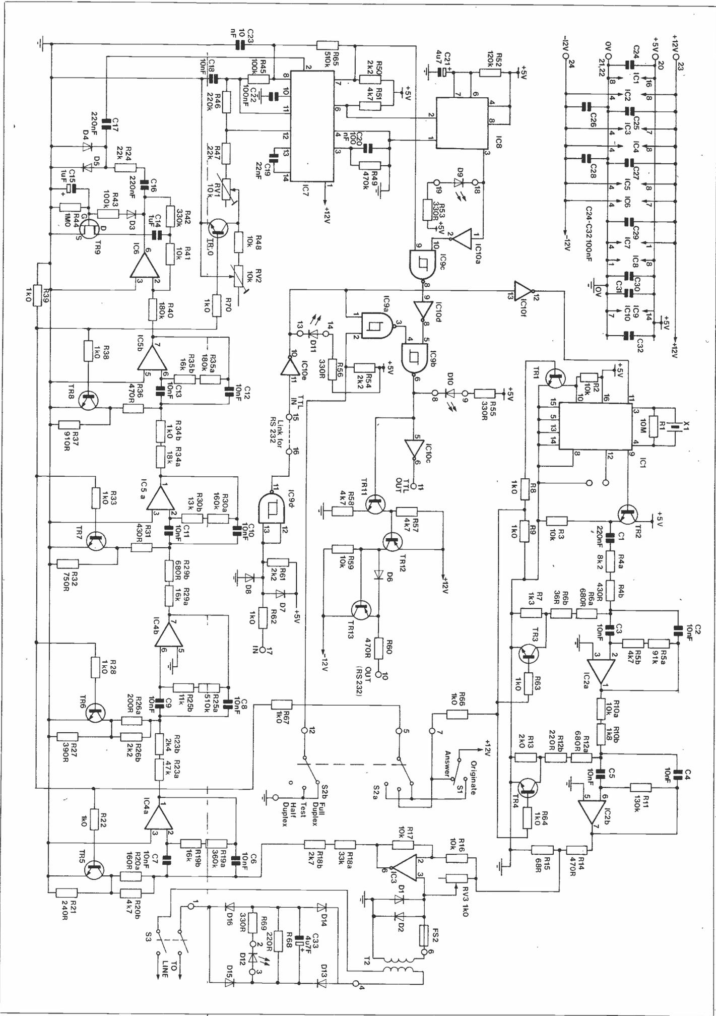
Figure 3. Modem main cct diagram
