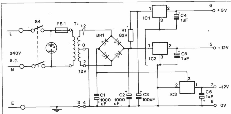
Figure 4. PSU circuit diagram
