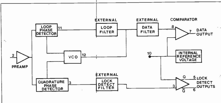
Figure 2. XR2211 block diagram
